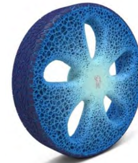
Michelin's Vision concept tire contains material composition, porosity, and colour gradients Source [21]
